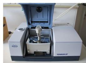
Identification via ATR-FTIR spectroscopy [Tensor 37, Bruker]
