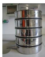
Size fractionation by sieving [2500  $\mu\text{m}$ , 500  $\mu\text{m}$ , 315  $\mu\text{m}$ ]
