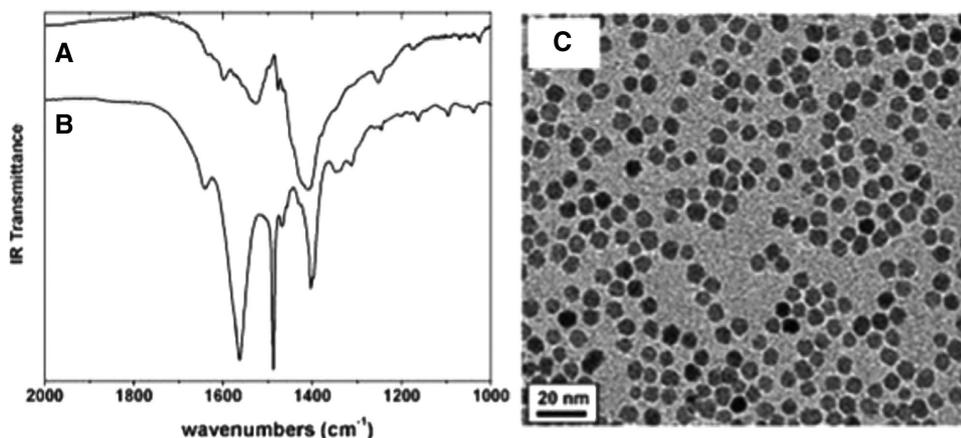
**Figure 12.** (A) Infrared spectrum of the as-synthesized hydrophobic 6 nm  $\text{Fe}_3\text{O}_4$  NPs, (B) infrared spectrum of tetramethylammonium 11-aminoundecanoate-coated 6 nm  $\text{Fe}_3\text{O}_4$  NPs, and (C) TEM bright field image of the 6 nm  $\text{Fe}_3\text{O}_4$  NPs (scale bar: 20 nm) in (B) deposited from water dispersion on amorphous carbon-coated copper grid. This figure is adapted with permission [143].
