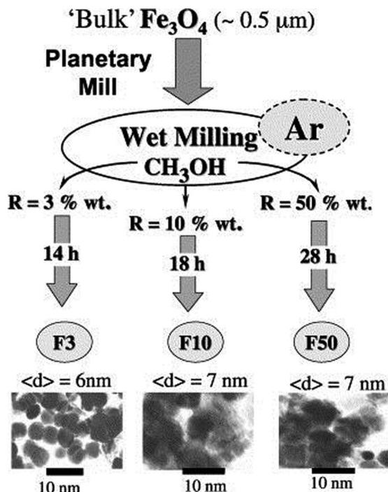
**Figure 3.** Schematic diagram of the ball milling experiment performed to obtain series of magnetite-based dispersions with different average crystallite sizes and concentrations (scale bar: 10 nm). This figure is adapted with permission [94].
