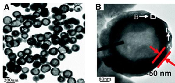
**Figure 9.** (A) TEM image of  $Fe_3O_4$  hollow spheres (scale bar: 200 nm). (B) Enlarged TEM image of an individual hollow sphere (scale bar: 80 nm). This figure is adapted with permission [133].
