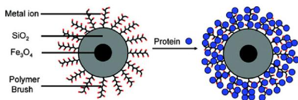
**Figure 19.** Schematic diagram of brush-modified materials and protein binding to these materials. This figure is adapted with permission [185].
