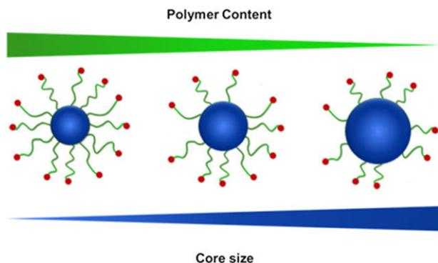
**Figure 5.** Decreasing amount of polymer used in a co-precipitation reaction results in superparamagnetic iron oxide NPs with similar hydrodynamic diameter. Larger iron oxide core size and less polymer in the outer shell. This figure is adapted with permission [121].
