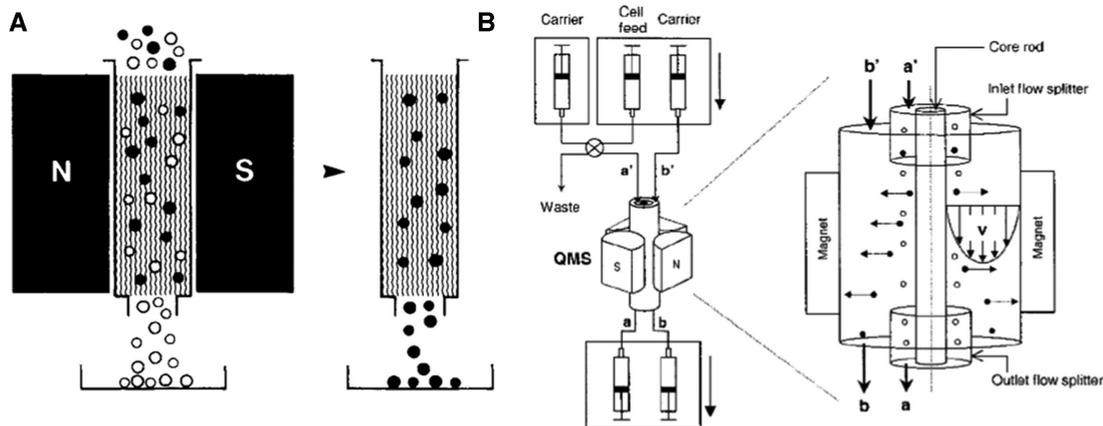
**Figure 17.** Conventional magnetic-activated cell sorting platform (A) standard quadrupole magnetic flow sorting and (B) deflection of magnetic moieties within a continuous stream flow stream. This figure is adapted with permission [180].
