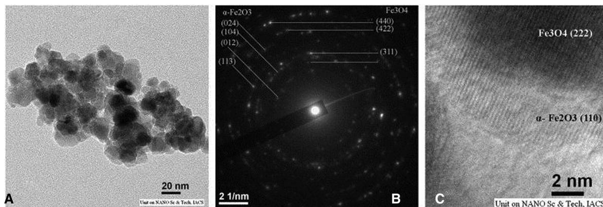
**Figure 4.** (A) Transmission electron micrograph for a specimen subjected to a milling operation for 6 h (scale bar: 20 nm). (B) Electron diffraction pattern obtained from Figure 4(A). (C) High resolution electron micrograph for a specimen grinding for 6 h (scale bar: 2 nm). This figure is adapted with permission [95].
