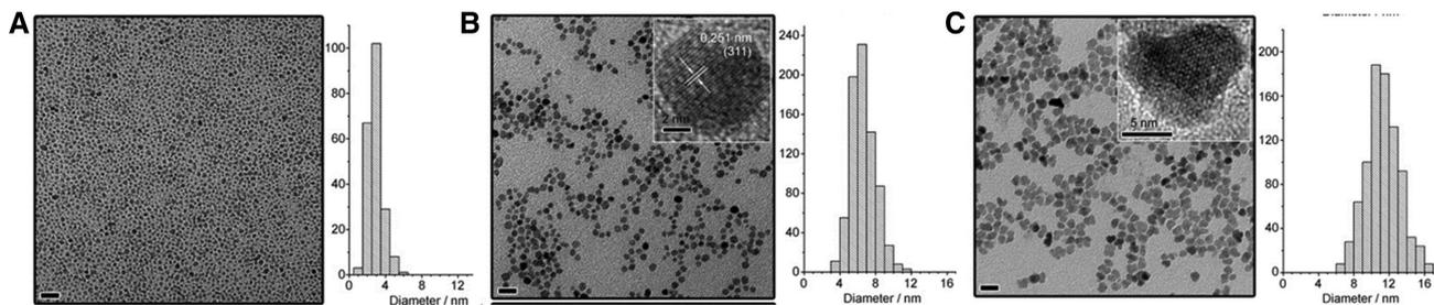
**Figure 8.** Representative TEM images and the corresponding measured size distributions of  $Fe_3O_4$  nanocrystals with an average diameter of (A) 2.9 nm, (B) 6.6 nm, and (C) 11.3 nm, respectively (scale bar: 20 nm). This figure is adapted with permission [131].
