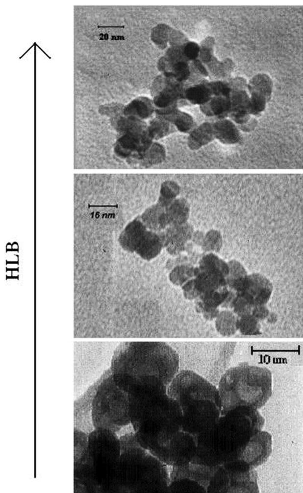
**Figure 10.** TEM images of prepared iron oxide NPs. The effect of HLB of the surfactant on the morphology of the samples was shown (scale bars: 20, 15, and 10 nm, respectively). This figure is adapted with permission [134].
