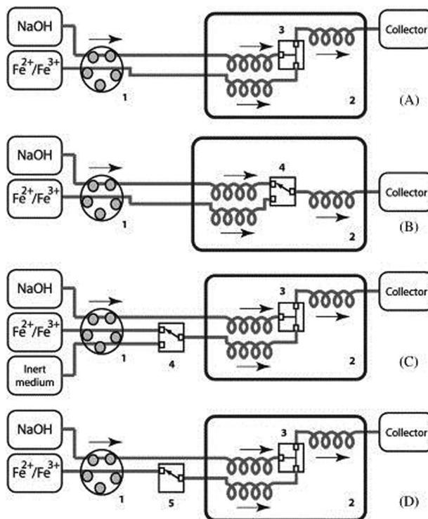
**Figure 11.** Different flow-injection schemes: (A) continuous injection; (B) flow segmentation by injection of reagents in turn; (C) flow segmentation with an inert medium; (D) flow segmentation by injection of one reagent in continuous flow of second reagent. (1) multi-channel peristaltic pump; (2) Thermostat; (3) t-injector; (4) computer-operated switching valve; (5) Computer-operated on-off valve. Helices indicate thermostated capillaries. This figure is adapted with permission [115].
