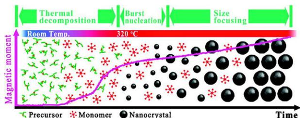
**Figure 7.** Effect of reaction temperature and reaction time on size, morphology and magnetic properties of iron oxide. This figure is adapted with permission [125].
