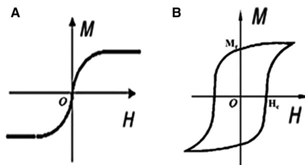
**Figure 1.** (A) Schematic magnetization loops of an ensemble of superparamagnetic particles and (B) ferromagnetic particles. This Figure is adapted with permission.
