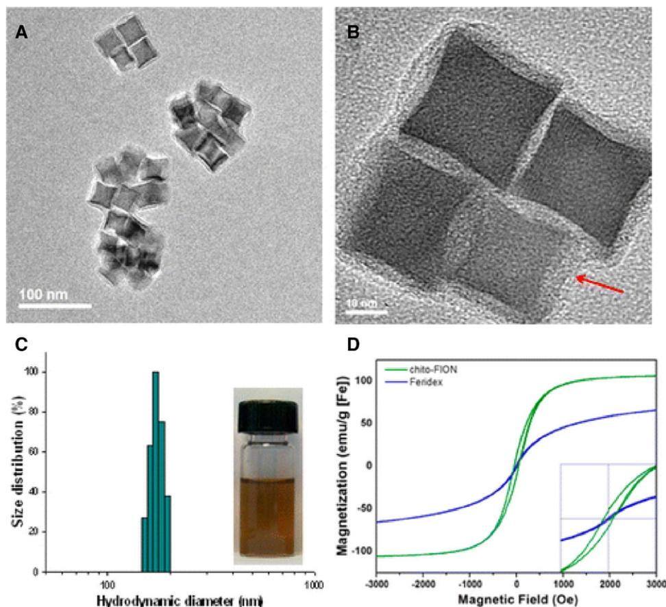
**Figure 13.** (A–B) TEM images of Chito-FIONs (red arrow indicates the presence of the polymer coating layers (scale bars: 100 nm and 10 nm, respectively). (C) Hydrodynamic diameters of Chito-FIONs in phosphate-buffered saline solution. Inset: Photograph showing the aqueous dispersion of Chito-FIONs. (D) Field-dependent magnetization curves of Chito-FIONs and Feridex. This Figure is adapted with permission [152].
