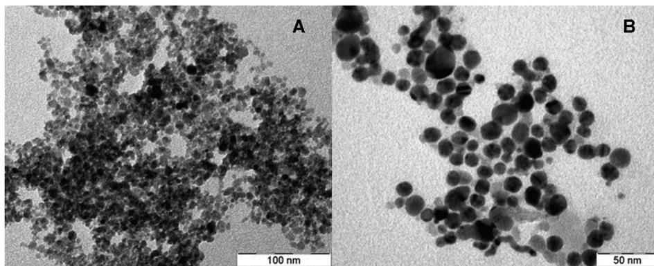
**Figure 15.** TEM images of (A) Magnetite NPs (scale bar: 100 nm) and (B) NPs of Fe<sub>3</sub>O<sub>4</sub>@Ag (scale bar: 50 nm). This figure is adapted with permission [164].
