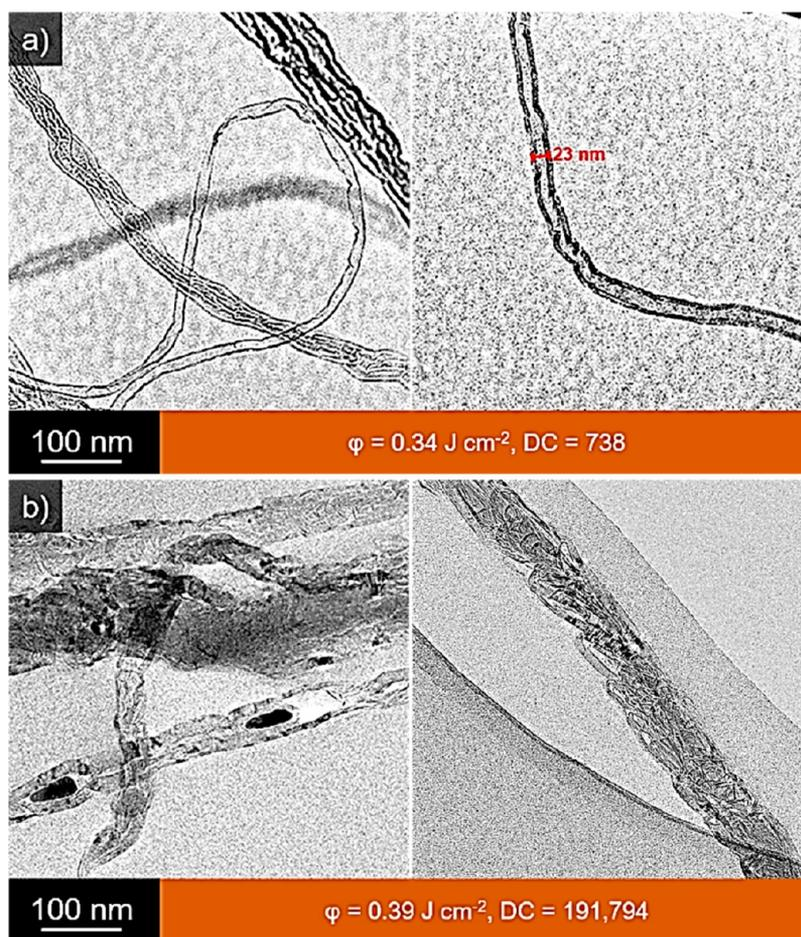
Figure 5. TEM images of (a) VA-CNTs and (b) CF-CNTs. (a) Width of the VA-CNTs match the c-NP size.  $\phi = 0.34 \text{ J cm}^{-2}$ , DC = 738. (b) CF-CNTs contain multiple c-NPs.  $\phi = 0.39 \text{ J cm}^{-2}$ , DC = 191,794.
