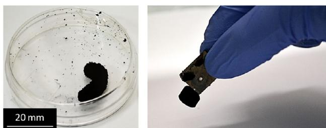
**Figure 9.** Photography of a CF-CNT bundle. The left image shows a CNT bundle, grown on a cauliflower catalyst field ( $\varphi = 0.72$  J cm<sup>-2</sup>, DC = 191,794). The size of the bundle is about 20 mm. On the right side, a piece of such a CNT bundle is attracted by a samarium–cobalt magnet.
