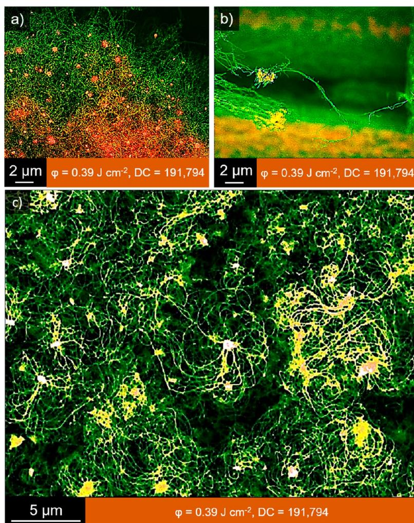
**Figure 6.** CF-CNTs with entrapped metal clusters. Carbon structures are pictured in green, whereby metallic catalysts are illustrated red/yellow. (a, b) Overlay of secondary and backscattered electron detectors. (c) Secondary electron image.  $\phi = 0.39 \text{ J cm}^{-2}$ , DC = 191,794.
