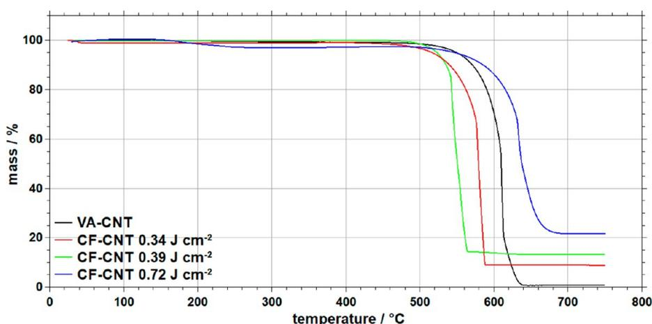
**Figure 8.** Thermogravimetric analysis (TGA) of VA-CNTs and CF-CNTs. VA-CNT catalysts:  $\phi = 0.34 \text{ J cm}^{-2}$ , DC = 738. CF-CNT catalysts:  $\phi = 0.34 \text{ J cm}^{-2}$ ,  $0.39 \text{ J cm}^{-2}$  and  $0.72 \text{ J cm}^{-2}$ , DC = 191,794. The higher the fluence applied, the higher the contained metal content is. (see also Figure S2).
