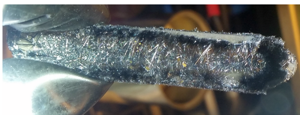
Figure 1. Single crystals of 1 grown on the walls of a corundum crucible.
