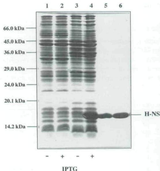
**Fig. 6.** Overproduction and purification of the H-NS protein. Cultures of strain BL21 (pPD1, vector plasmid; lanes 1 and 2) and strain BL21 (pPD3, *hns*<sup>+</sup>; lanes 3 and 4) were grown in the absence (-) or presence (+) of IPTG. Total cell extracts were prepared, and the proteins were electrophoretically separated on a 15% SDS-polyacrylamide gel. Lanes 5 and 6: purified H-NS protein (4  $\mu$ g in lane 5 and 8  $\mu$ g in lane 6).
