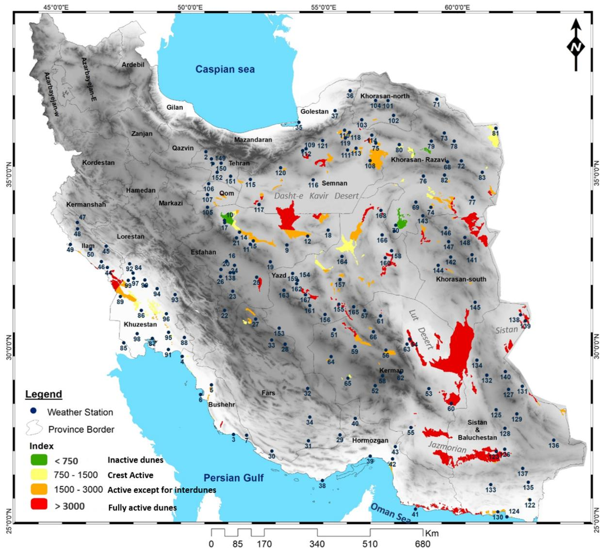
Fig.12. Sand dune activity in Iran based on the Modified Lancaster Index (MLI).
