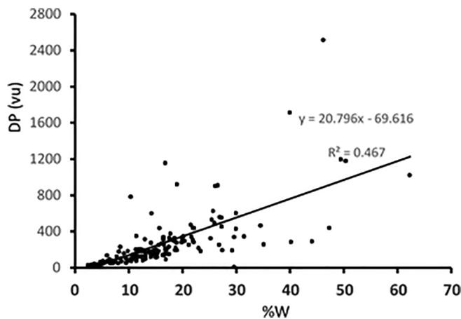
**Fig. 10.** Relation between sand drift potential (DP) and the percent time wind above transport threshold (W) in selected meteorological stations in Iran.
