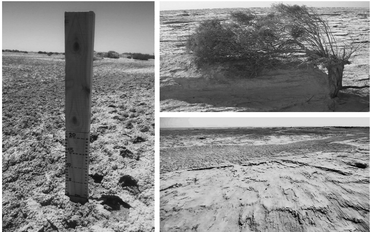
Fig. 3. Graduated erosion pin (left) and indicators of the wind energy in the Baringak lake (right).
