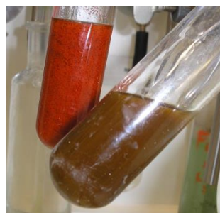
Scheme 3. Synthesis of pyrrolidinium hexasulfides from trimethylsilylthiolates (left), and bis( N -butyl- N -methyl-pyrrolidinium)hexasulfide precipitating during the reaction (red).
