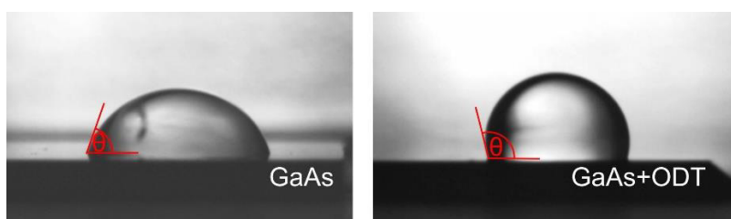
Fig. 1: Contact angle of GaAs surface after etching (left, \theta \approx 70^\circ ) and with ODT modification (right, \sim 105^\circ ).
