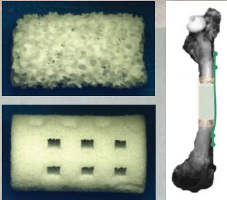
**FIGURE 1.** 3D-CALCIUM ALKALI PHOSPHATE SCAFFOLDS FOR BONE TISSUE ENGINEERING
