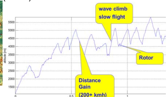
Figure 5 Barogram of Wave Track Flight. Predicted wind field showed a North-Westerly direction. This is consistent with Figure 3. Wind speeds were predicted above 50 km/h and a positive, i.e. increasing, wind shear was predicted and encountered (data not shown).
